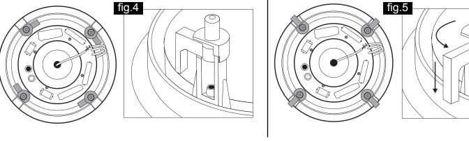
**6.** The bezel (with driver) attaches to the bracket via four plastic mounting clamps on the back of the bezel that swivel to "sandwich" the drywall between the bezel frame and the clamps (fig.4). First rotate the mounting clamps counterclockwise so that the body of the bezel can slide through the mounting bracket. Exercise caution not to damage the driver.
